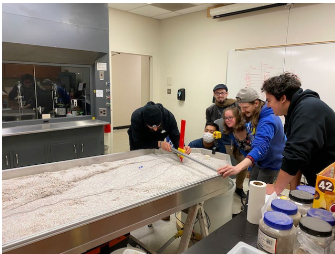
Students in GEOL 3080 Geomorphology measuring channel sinuosity on the stream table.
