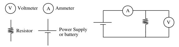
The connecting lines represent wires.
