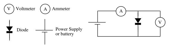
CAUTION: Obtain the maximum current rating of the diode from your instructor and do not exceed it; to do so would damage the diode.
